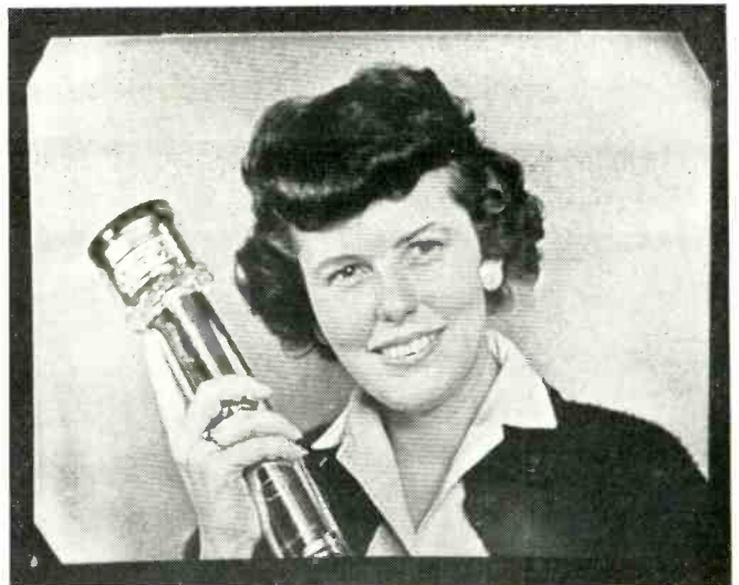
reduction in this problem with the new field mesh image orthicon. Note also the reduction of edge-effect at the fingers and collar.
