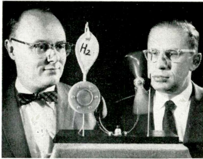
Fig. 14: Fuel cell produces electricity directly from gaseous fuel while GE Scientists, Drs. L. W. Niedrach (l) and W. Thomas Grubb look on. Fuel (hydrogen) is in balloon marked "H 2 ." Water is by-product.
