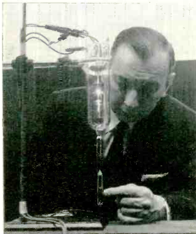
Fig. 23: Dr. J. W. Coltman, Mngr., Electronics and Nuclear Physics Dept., Westinghouse Research Labs., demonstrates experimental thermionic generator. Capsule at base of tube holds Cesium used for neutralizing the space charge effect.
