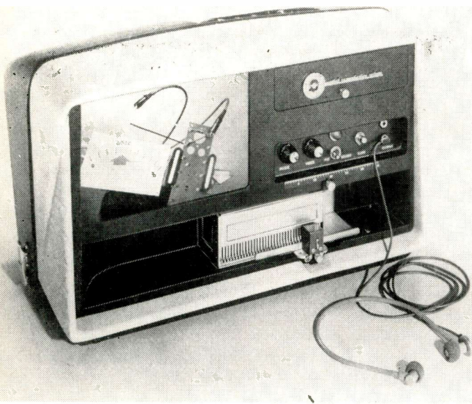
Audio-visual unit contains both a 35mm slide projector and a synchronized sound tape playback mechanism.
