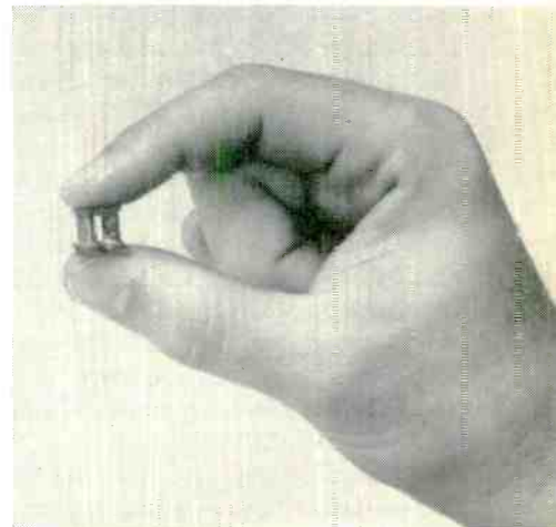
Fig. 24: Thermoelectric unit built by Materials Electronic Products Corp., Trenton, N. J. Fig. of Merit (p-type) is 4 to 4.5 \times 10^{-3} ; (n-type) is 2.7 to 3 \times 10^{-3} . This is a cooling unit. Generator elements are similar in physical structure.
