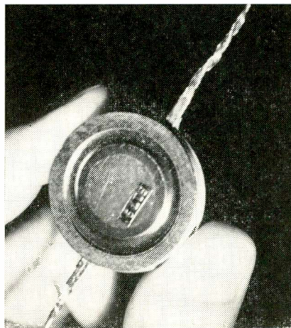
Vapor Thermionic Converter. Device uses Cesium gas to help overcome space-charge effect between cathode and anode. Power density is 2 w/cm 2 ; efficiency (operating at 1300°C) is from eight to twelve per cent.
